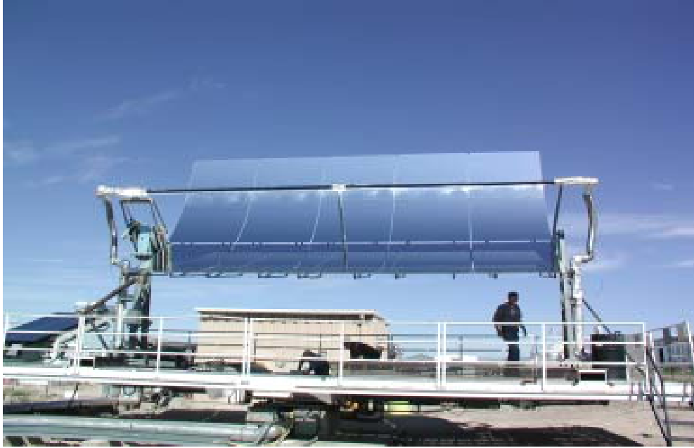
Figure 5.1 AZTRAK rotating test platform at SNL. An LS-2 type collector module is shown installed on the platform.
