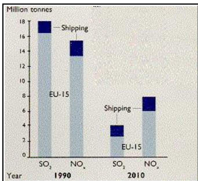
Figure 3.48 Development of \text{SO}_2 and \text{NO}_x emissions from land-based sources and shipping assuming the later to stay outside stricter regulations (picture from "Cleaner Shipping", 1997)
