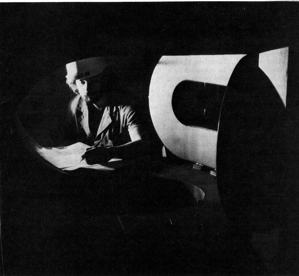
The tandem mirror machine at Lawrence Livermore Laboratories. On the left is the interior of the central tube. A technician is tightening down the titanium "getter" wires; after each plasma pulse titanium is evaporated from these wires and deposited on the vacuum chamber walls to cover adsorbed impurities. The large coils provide a focussing field for the plasma beam. It is this part of the machine that could be surrounded by a blanket of fertile material to produce fissile isotopes for use in ordinary fission power plants. On the right is a "beam's eye view" of one of the two magnetic mirrors that are at the ends of the tube shown at left. Note that the main coil for the mirror is shaped like the seam of a baseball. (Both photos by David Proffitt, Lawrence Livermore.)
