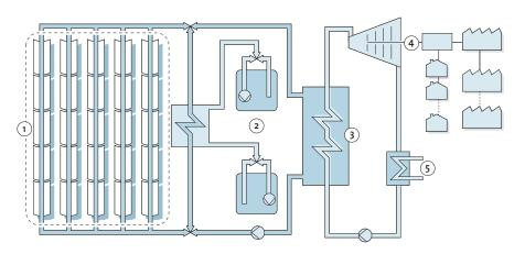
1. Solar field, 2. Storage, 3. Heat exchanger, 4. Steam turbine and generator, 5. Condenser
