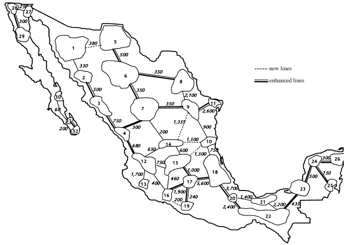
Figure 4: Planned changes to the transmission network by 2005
