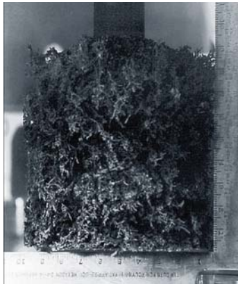
Figure 7. Dendritic uranium deposit on electrorefiner cathode.
