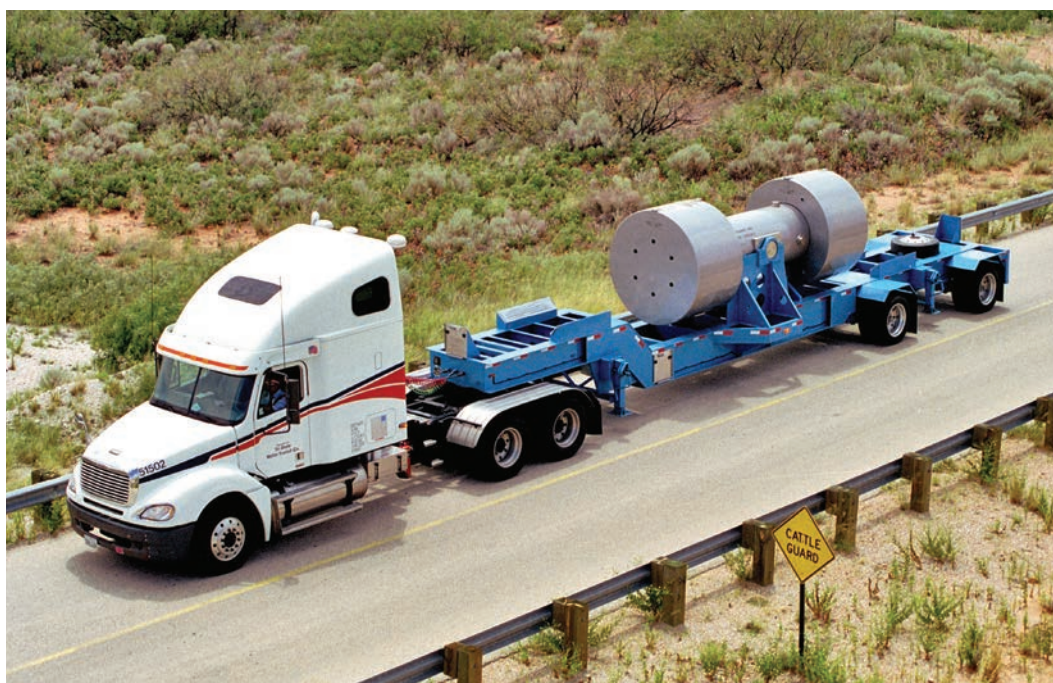
FIGURE 3.6. A RH72-B cask containing a load of high-activity waste contaminated with transuranics en route to the Waste Isolation Pilot Plant near Carlsbad, New Mexico. SOURCE: https://flic.kr/p/omVazd
