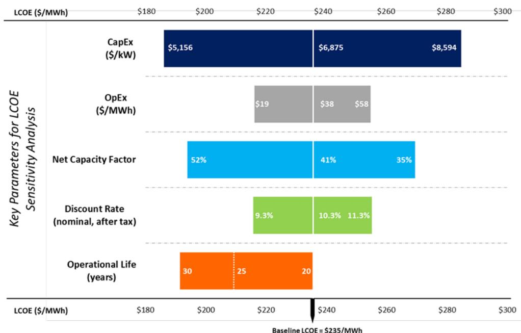
**Figure ES6. Floating offshore wind plant assumptions and ranges for key LCOE input parameters**
