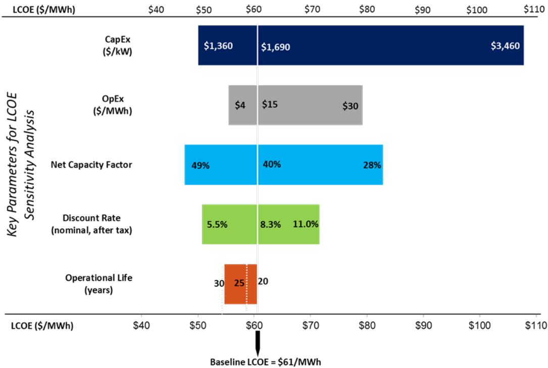
**Figure ES4. Land-based wind plant assumptions and ranges for key LCOE input parameters**
