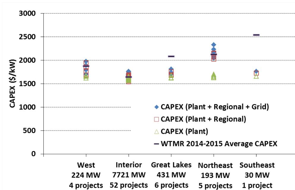
**Figure 10. CapEx estimated for locations where projects were installed in 2015 including the wind plant, regional cost increment, and grid connection cost increment**
