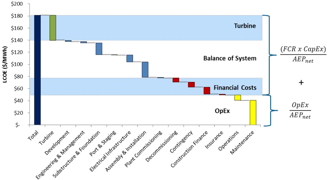
**Figure 16. Cost breakdown for the 2015 fixed-bottom offshore wind reference project**
