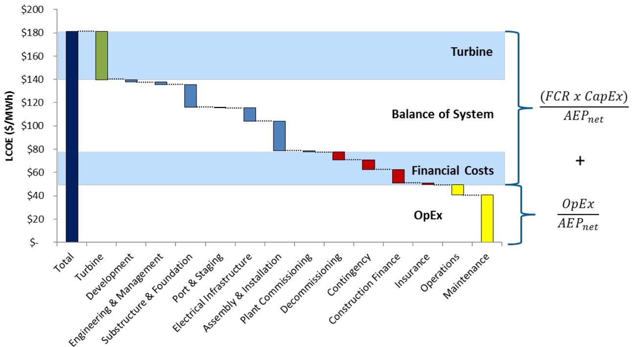
**Figure 17. Cost breakdown for the 2015 floating offshore wind reference project**
