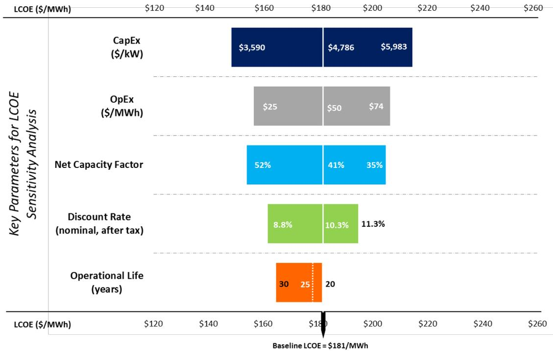
**Figure 18. Sensitivity of fixed-bottom offshore wind LCOE to key input parameters**
