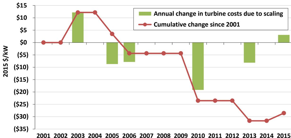
Figure 28. Impact of scaling on wind turbine costs
