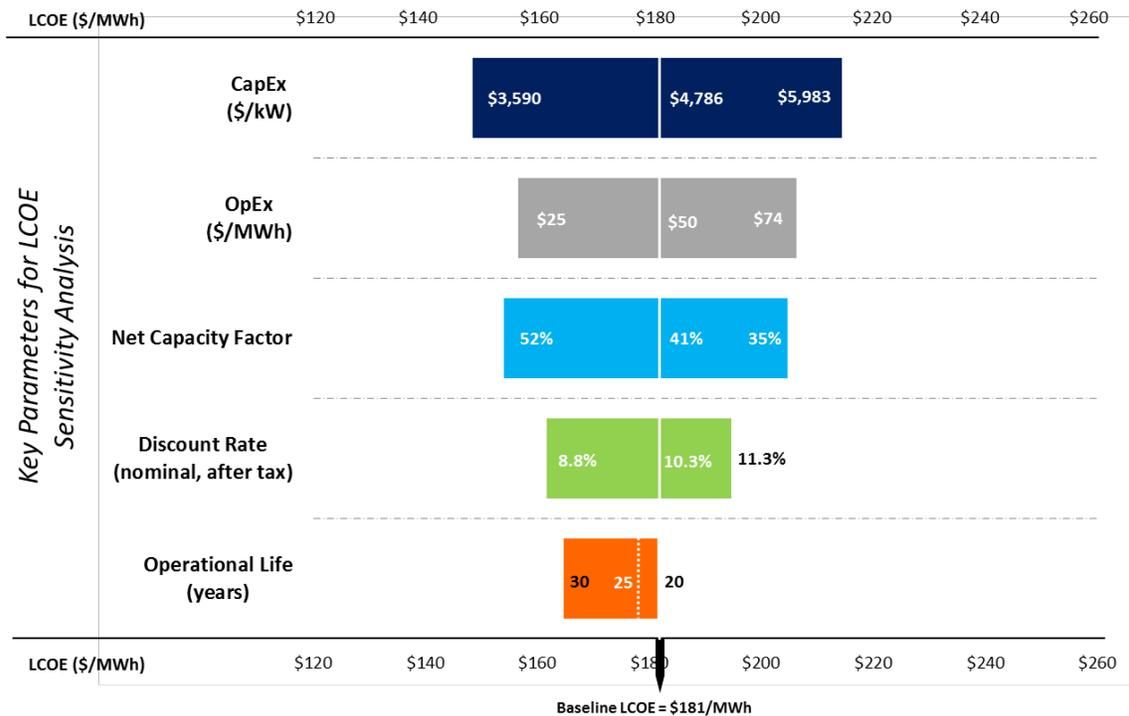
**Figure 19. Sensitivity of floating offshore wind LCOE to key input parameters**
