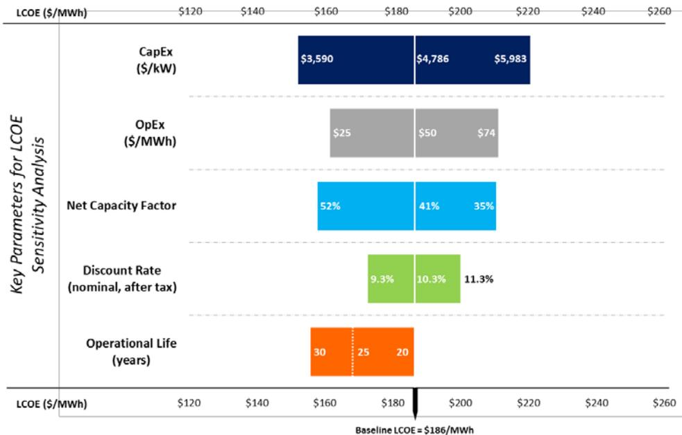
**Figure ES5. Fixed-bottom offshore wind plant assumptions and ranges for key LCOE input parameters**
