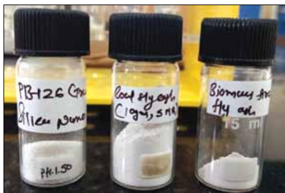
Fig. 10.29: Extracted SiO 2 Nano particles from Rice straw (PB 126), Industrial coal fly ash, and Biomass fired fly ash
