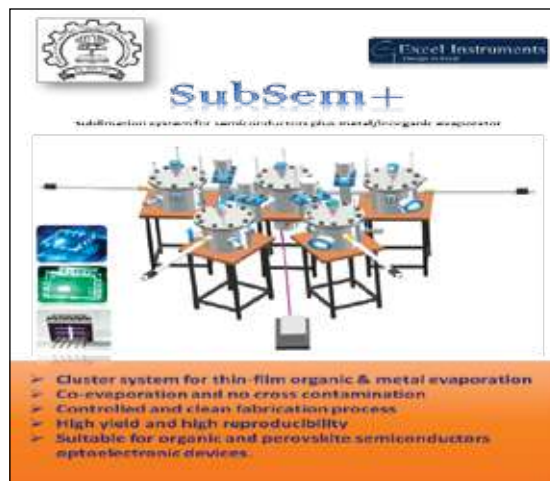
Fig. 7.5: Schematic of in-house developed cluster tool for making highly reproducible perovskite optoelectronic devices.
