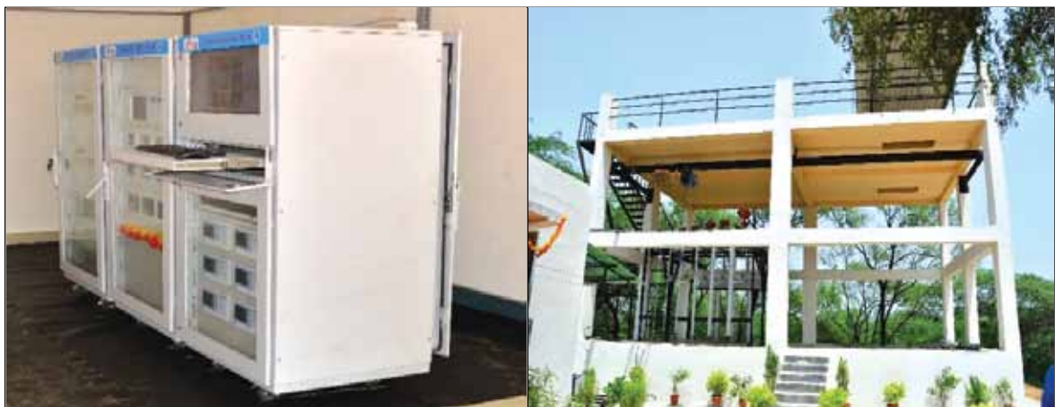
Fig. 10.11: Solar Water Pump Test facility for up to 50 hp at NISE
