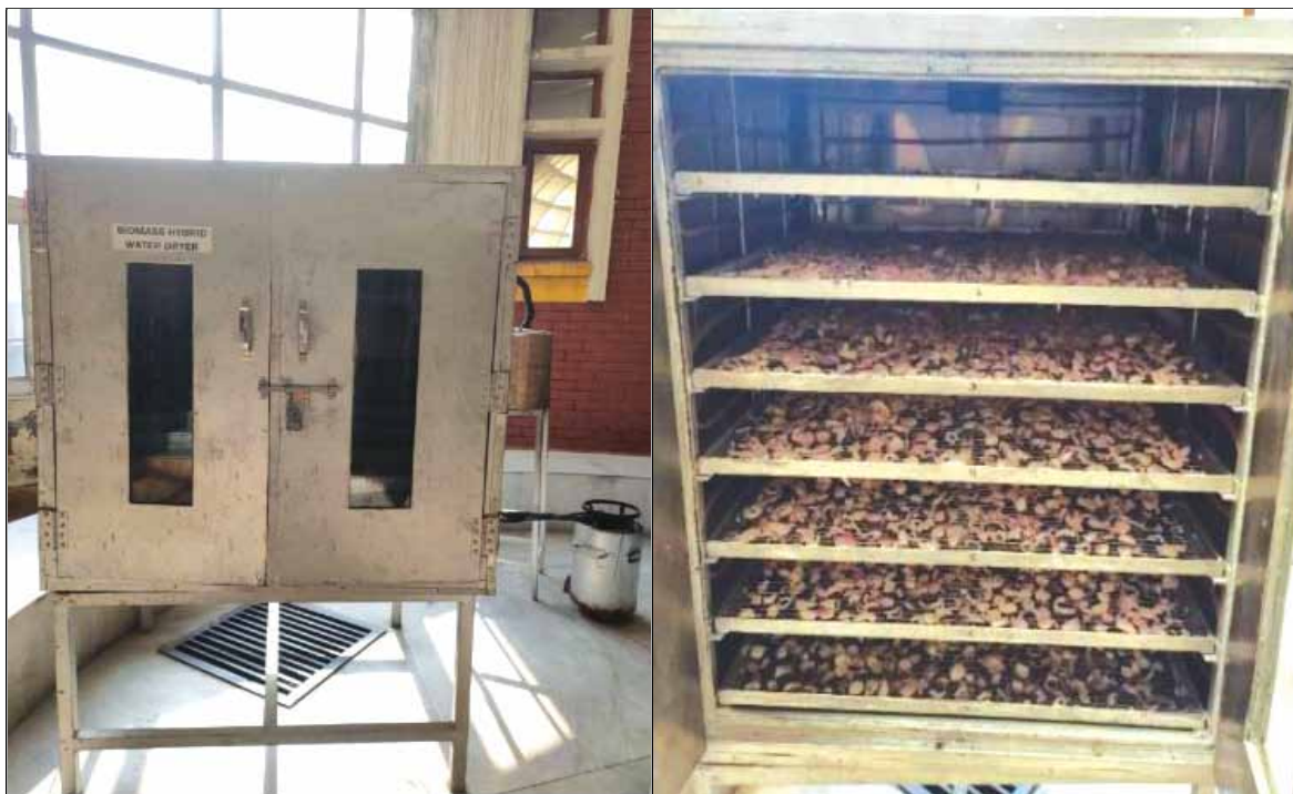
Fig. 10.25: Biomass Hybrid Dryer and drying of Onion flakes using bioenergy
