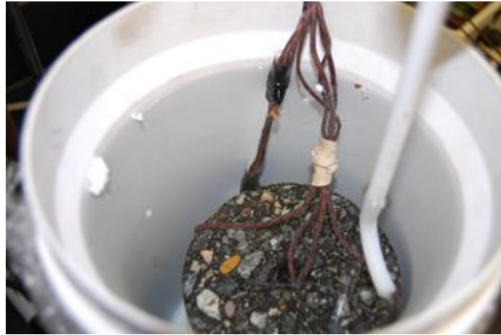
Figure 43. Specific heat laboratory testing setup
