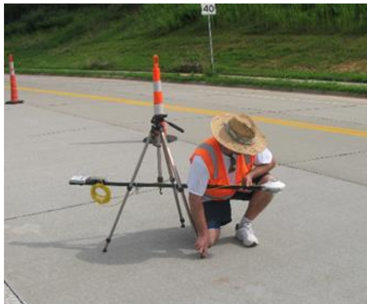
Figure 34. Albedometer mounting during city field testing
