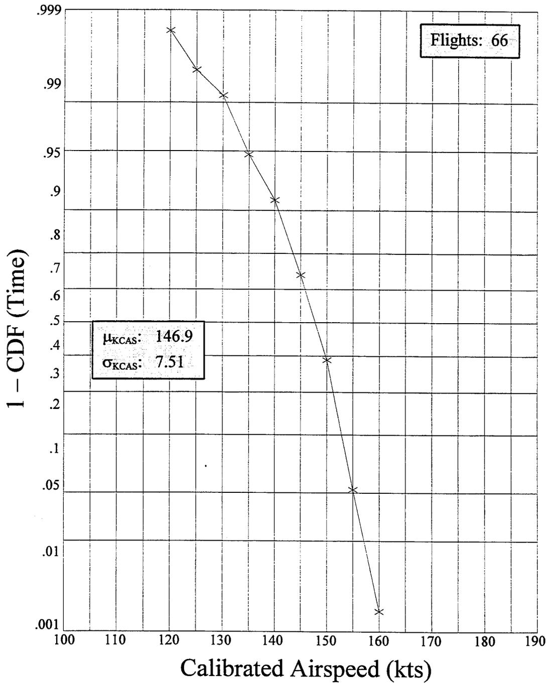
FIGURE 26. CUMULATIVE DISTRIBUTION OF CALIBRATED AIRSPEED AT FLAP DETENT 40
