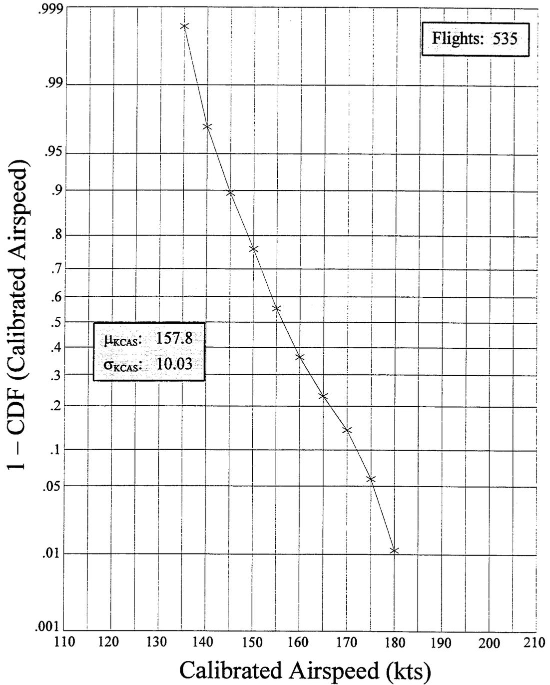
FIGURE 25. CUMULATIVE DISTRIBUTION OF CALIBRATED AIRSPEED AT FLAP DETENT 30
