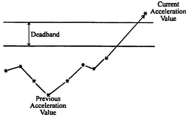
FIGURE 6B. CURRENT ACCELERATION VALUE PASSES THROUGH DEADBAND
