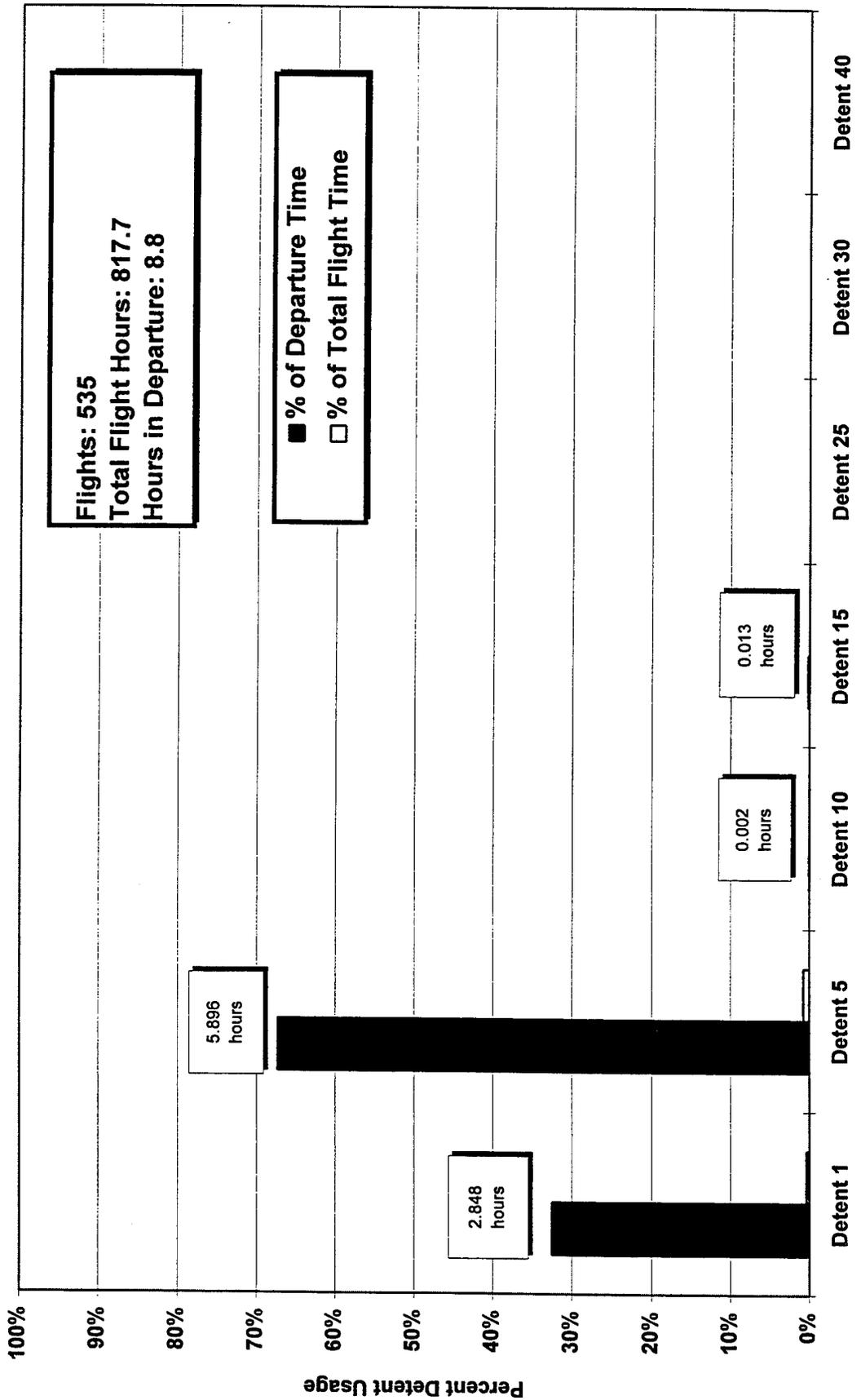
FIGURE 18. FLAPS USAGE BY FLAPS DETENT DURING DEPARTURE
