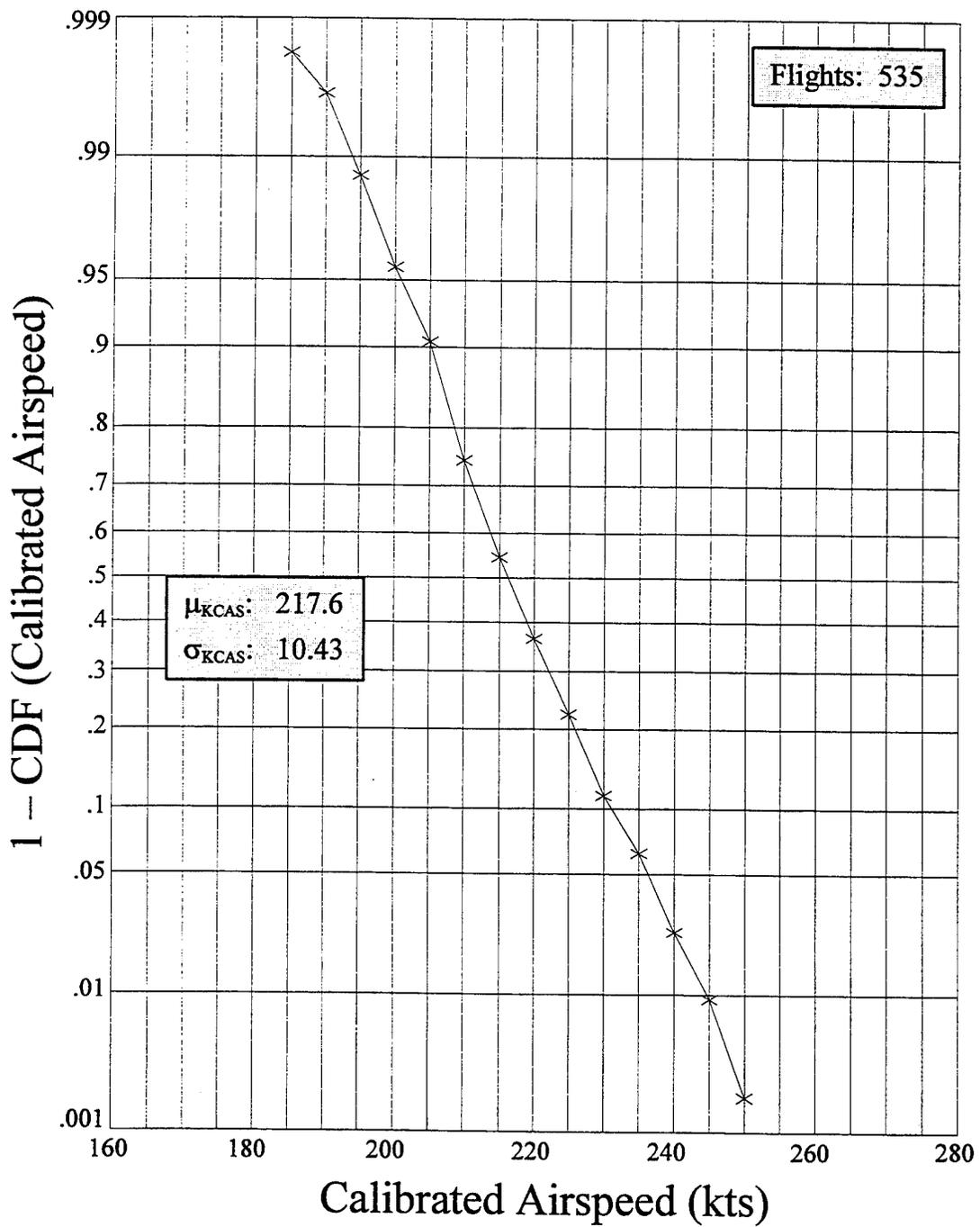
FIGURE 20. CUMULATIVE DISTRIBUTION OF CALIBRATED AIRSPEED AT FLAP DETENT 1
