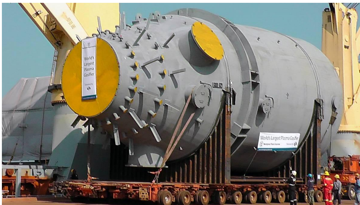
Fig.4. The largest plasma reactor in the world - 1000 tpd G65 WPC reactor before installation at Air Products’ location in Tees Valley, Northeastern England
