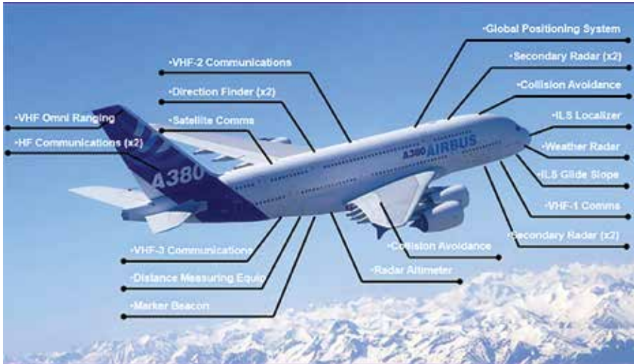
Figure 1.7. Airbus A-380 electronic systems. (Source: FAA)
