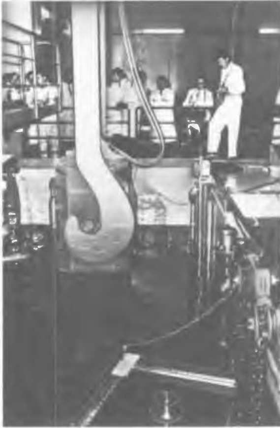
FIG.13. WAK pool receiving shipping cask.
