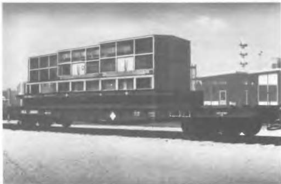
FIG. 12a IF-300 rail cask capable of holding 7 PWR or 18 BWR assemblies.
