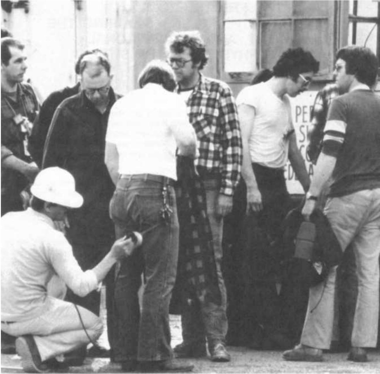
Hand-held "friskers" were used by TMI personnel to check plant workers for radiation.
