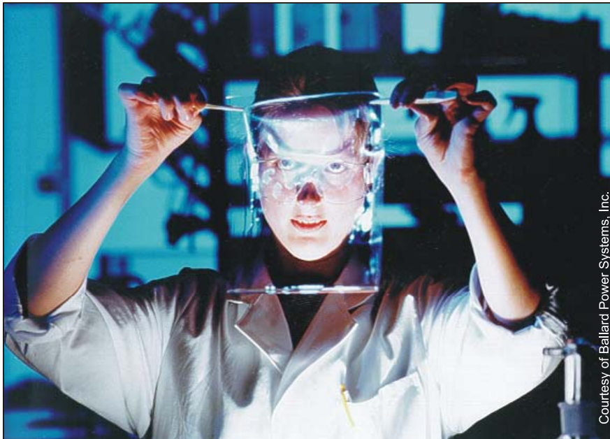
Figure 4-19 A Solid Electrolyte Membrane For Ballard's PEM Fuel Cells
