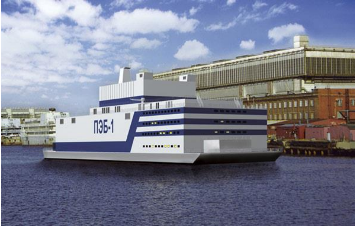
Figure 6. An artist's rendition of the Russian floating-barge nuclear power station. The unit can carry two KLT-50S icebreaker-type reactors, for 70 MWe, to a remote site. 51
