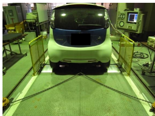
Figure 12: “i-MiEV” on the dynamo system
