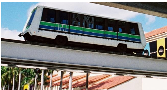
Automated guideway transit trains provide distributor or shuttle service without an on-board operator. The Miami-Dade County Metromover, a 4.4 mile long fully automated system, connects heavy rail stations and bus service with major destinations in downtown Miami, FL. Automated guideway transit data are included with other rail modes in Tables 36 and 39.
