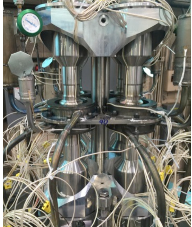
Figure 3.—Balance of plant hardware showing eight Haynes® 230® sodium heat pipes attached to a conduction plate that supplies heat to two Stirling engines and six Stirling thermal simulators.
