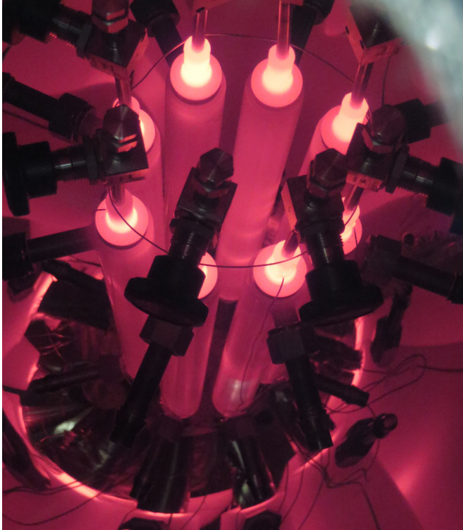
Figure 2.—Thermal prototype testing with Haynes® 230® sodium heat pipes radiating at over 800 °C to the vacuum chamber walls as seen through the chamber view port.
