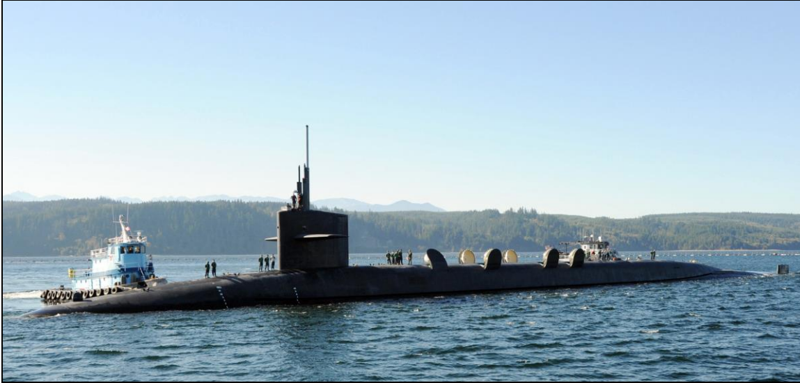
Figure 1. Ohio (SSBN-726) Class SSBN With the hatches to some of its SLBM launch tubes open
