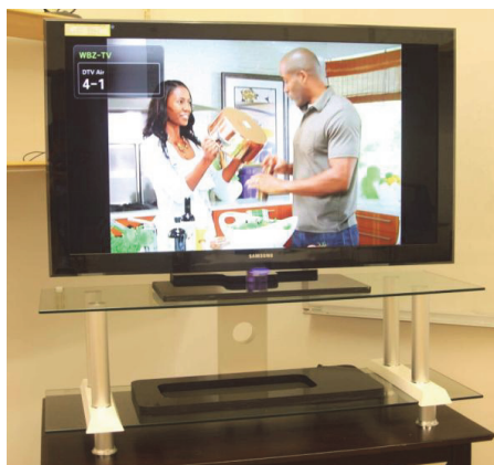
Figure 3: Photographs of highly resonant wireless power transfer systems used to wirelessly power and operate an LCD TV (~250 W supplied wirelessly) (left) and to wirelessly charge a battery in a smart phone (~5 W supplied wirelessly) (right).
