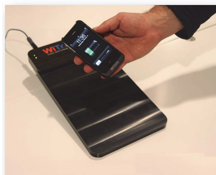
Figure 3: Photographs of highly resonant wireless power transfer systems used to wirelessly power and operate an LCD TV (~250 W supplied wirelessly) (left) and to wirelessly charge a battery in a smart phone (~5 W supplied wirelessly) (right).
