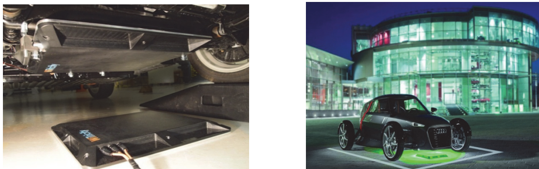
Figure 7: Photograph showing an application of HR-WPT for charging full electric and hybrid vehicles.
