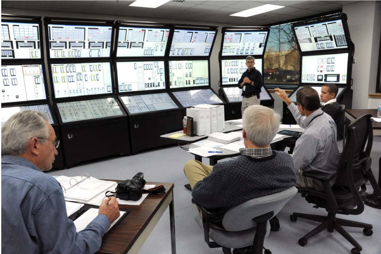
Figure 16. An operator workshop with a nuclear utility being conducted in the HSSL using the bench-board-style touch panel control bays.
