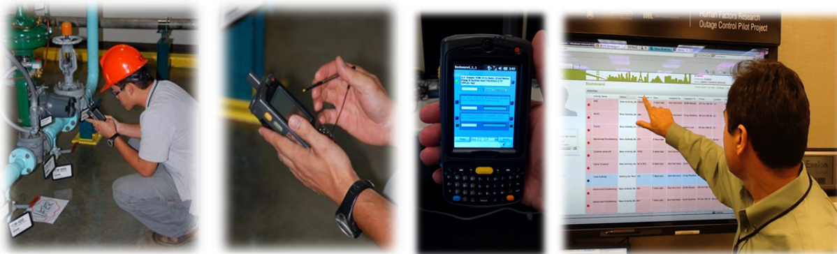
Figure 12. A nuclear power plant field worker performs his work using a portable, wireless, hand-held device developed for LWRS Program research instead of paper-based work packages.
