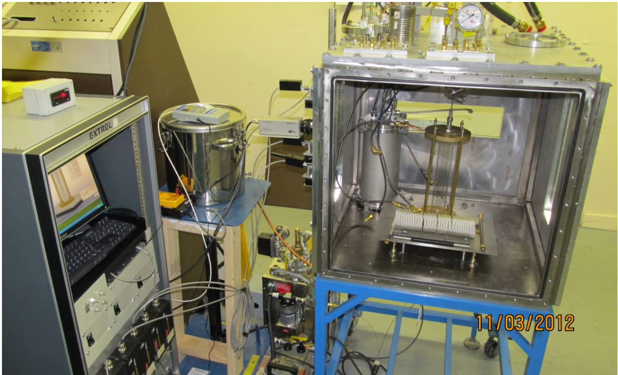
Figure 25. Oxidation Kinetics System (OKS) test chamber, steam generator, water reservoir and data acquisition system.
