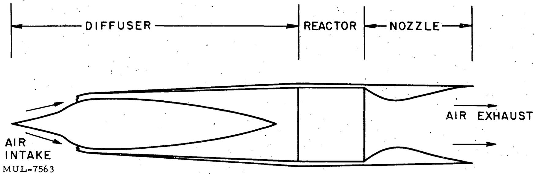
Fig. 1. Conceptual arrangement of a nuclear ramjet.
