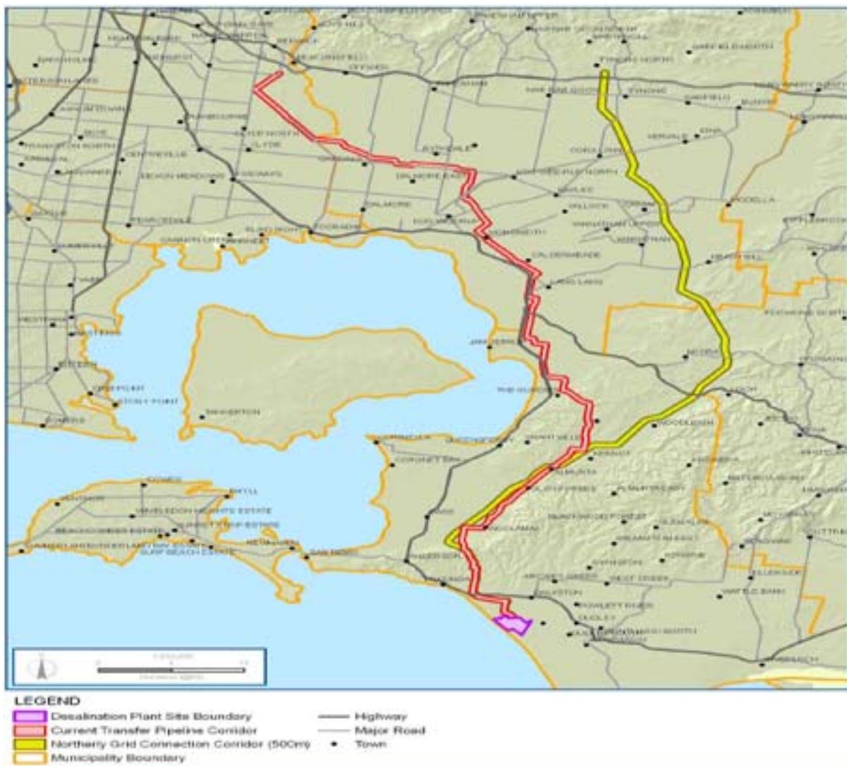
Figure 2: Transfer Pipeline and Power Supply Corridors
