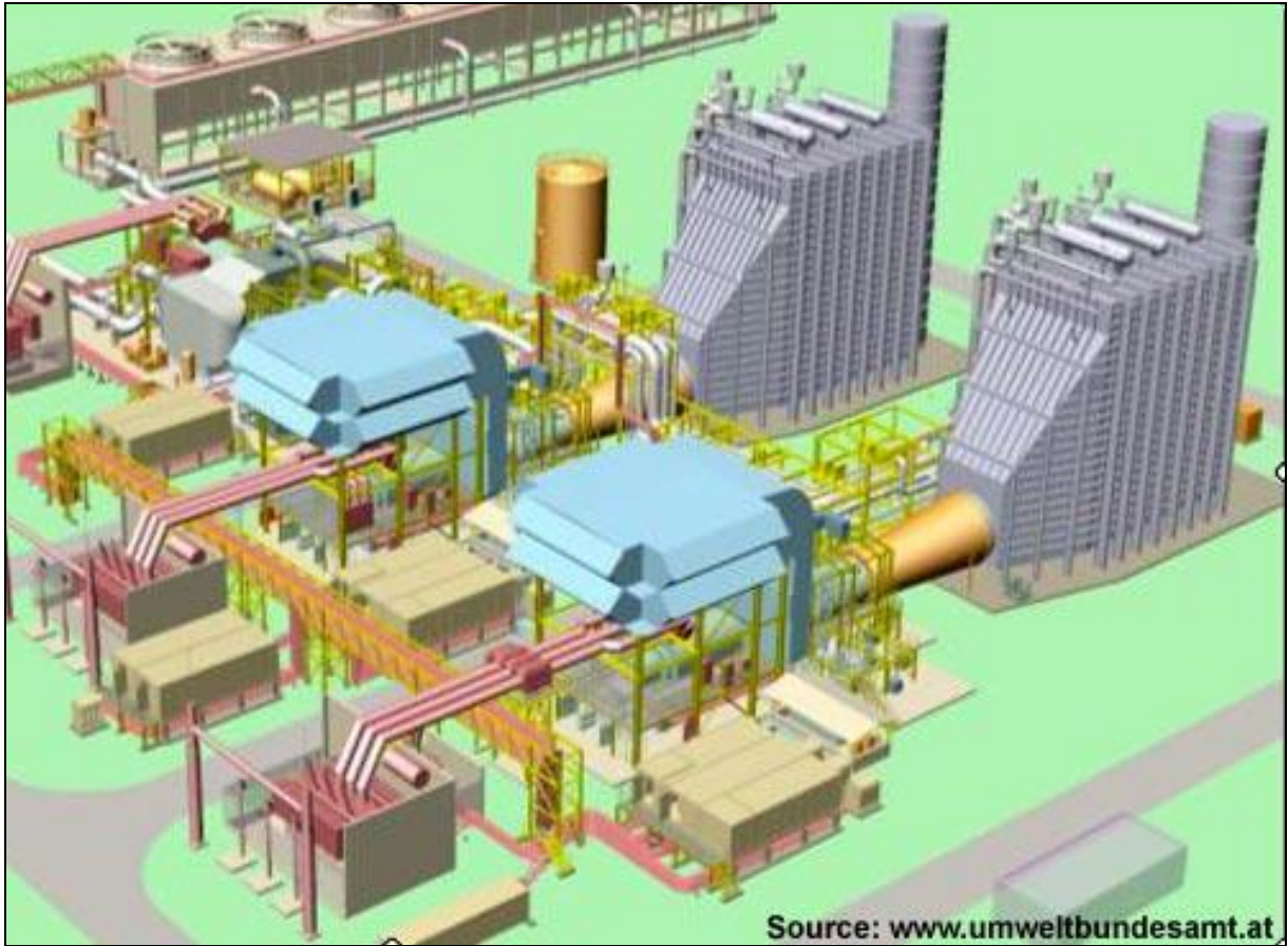
Figure C-4: Combined Cycle Power Plant General Arrangement
