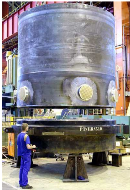
Figure 12 - Large Reactor Pressure Vessel (RPV) forgings with nozzles. (Courtesy of AREVA NP).
