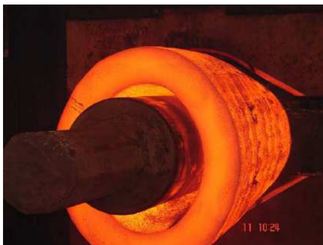
Figure 11 - Reactor Pressure Vessel (RPV) forging. (Courtesy of AREVA NP).
