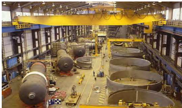
Figure 13 – Steam Generator fabrication at Babcock Energy Ltd. (now Doosan Babcock), Renfrew, for Sizewell B. (Courtesy of Doosan Babcock).
