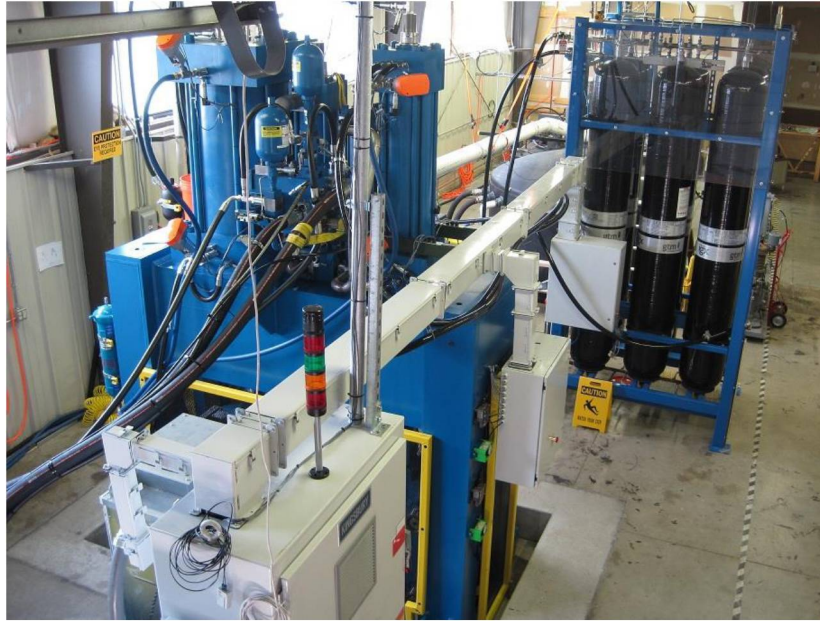
Figure 8: 40 kW Pilot unit at the original Lebanon, NH location, showing cylinders and air storage vessels (back right)
