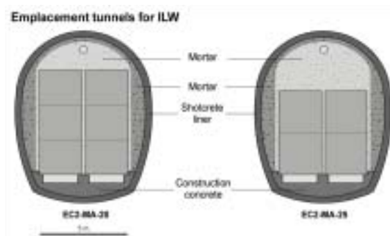
Cross-section of a typical conceptual design for a repository for large-volume containers of ILW using concrete-lined caverns (courtesy Nagra).
