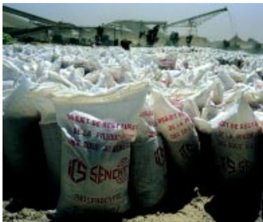
Bagging of phosphogypsum for use as a soil amendment. Darou-Khoudoss, Sénégal. (Industries Chimiques du Sénégal)
