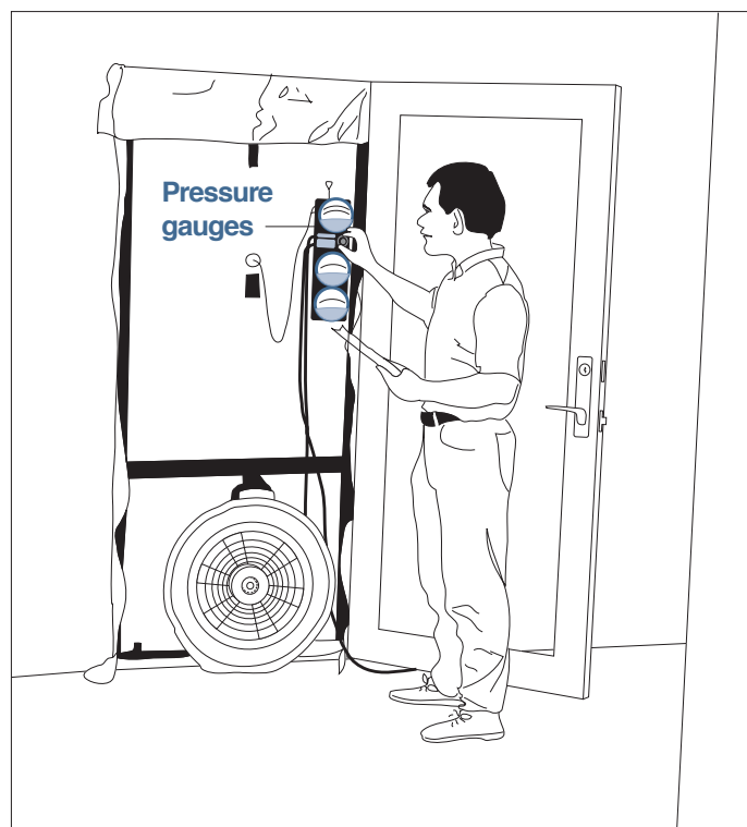
Figure 1-14 - Blower door for testing air leakage.
