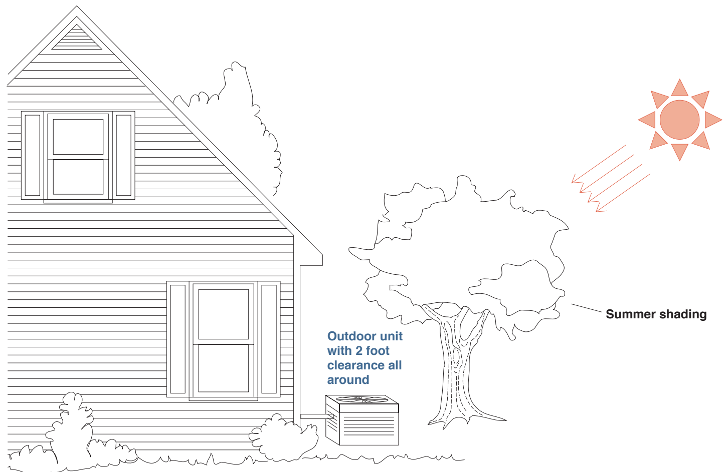
Figure 5-11 - Air conditioner unit with proper ventilation and sun protection
