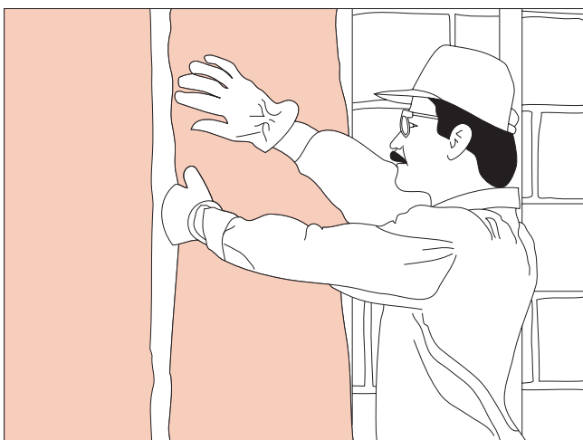
Figure 3-2 - Fiberglass batts are installed in open walls and floors. Wearing a dust mask, gloves, and goggles can help avoid irritation from fiberglass dust.
