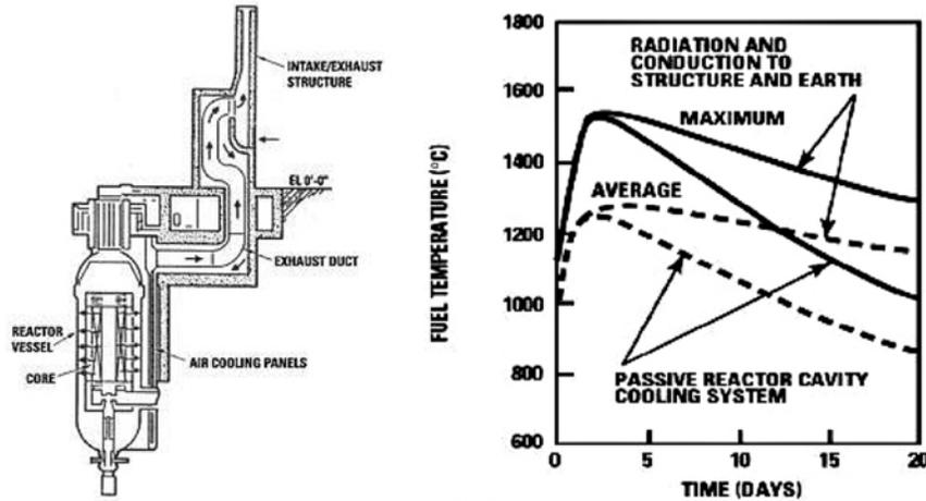
**Figure 2.5-3. GT-MHR Passive RCCS and Peak Accident Core Temperatures (Ref. 19)**
