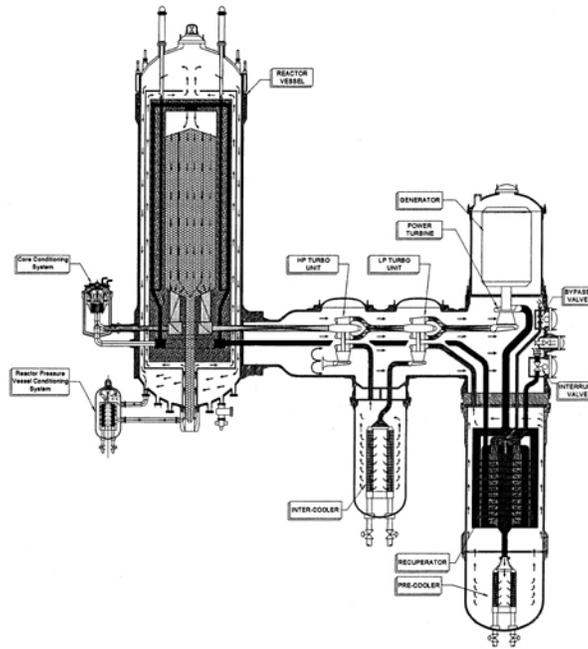
**Figure 4.2-3. The Pebble Bed Modular Reactor (PBMR) by PBMR (Pty.), Ltd. (Ref. 6)**
