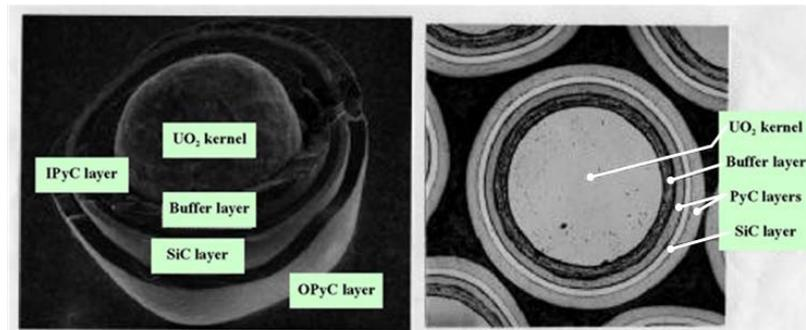
Figure 2.4-1. TRISO (Triple Isotropic) Coated Fuel Particle (Ref. 11)
