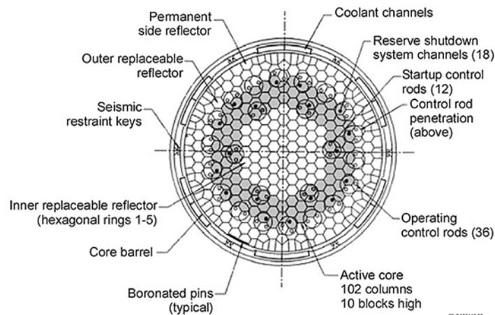
**Figure 2.2-1. The GT-MHR Reactor Core (Prismatic VHTR Reference Core) (Ref. 15)**
