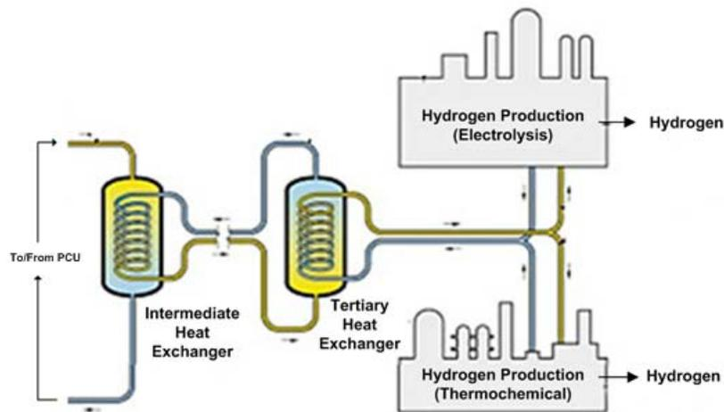
Figure 2.5-2. NGNP Secondary Heat Transfer Loop
