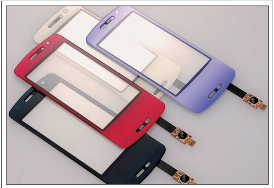
Fig. 7: Smartphone pro-cap touch-screen modules manufactured by Nissha Printing consist of a pro-cap sensor, a decorated cover lens laminated to the sensor and a controller mounted on the FPC (flexible printed circuit) that makes up the touch-screen connector tail. Source: Nissha Printing.
