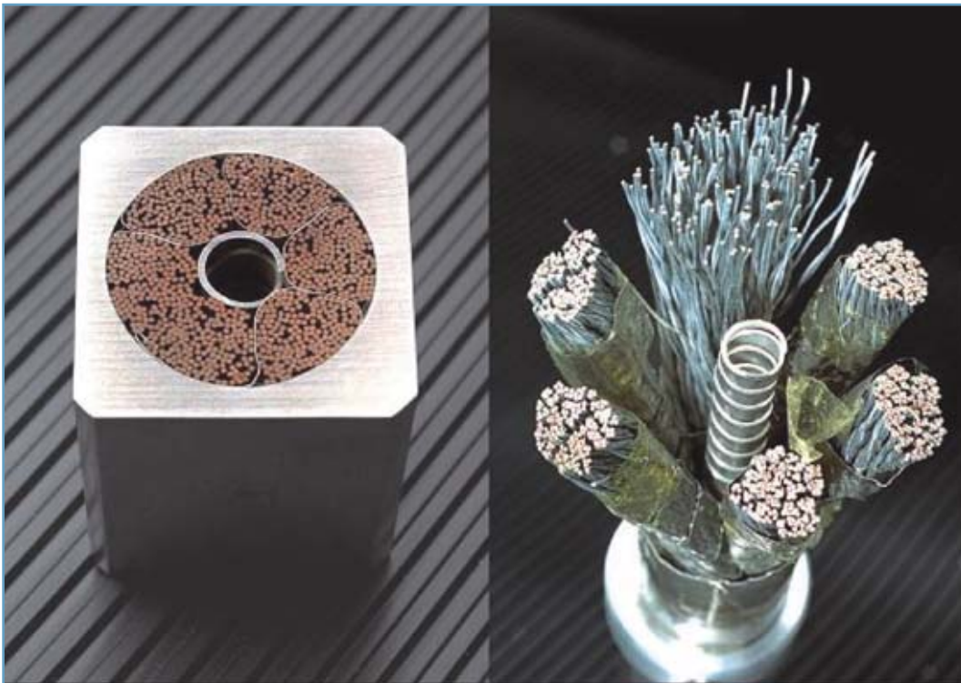
Figure 4. On the left, the CICC of the ITER's central solenoid model coil (51 mm x 51 mm, 40 kA); on the right, exploded view of the CICC of the model coil for the ITER's TF system (diameter 40.7 mm, 80 kA).
