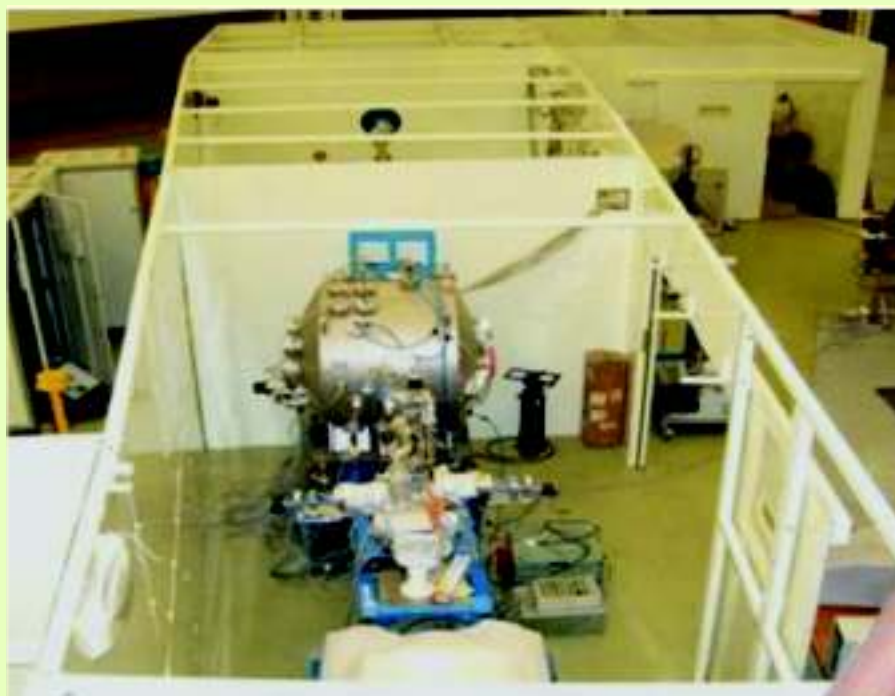
Indus-2 Synchrotron Radiation beam line with shielding hutch
