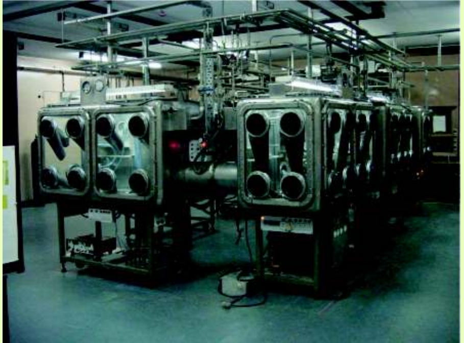
Glove box facility for fabrication of sodium bonded metallic test fuel pins
