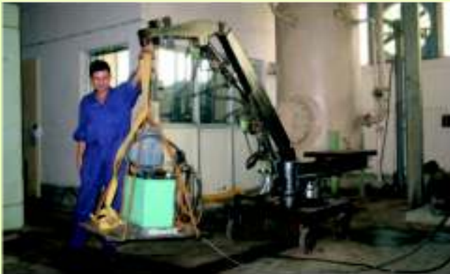
Hydraulic Balancer for handling heavy loads
