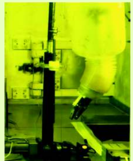
Non-destructive testing of the fuel inside the hot cell
