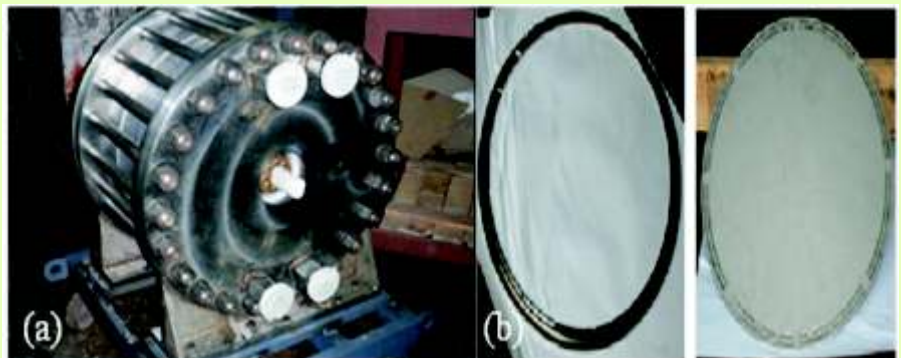
(a) 25-cell module assembly for the skid mounted Hydrogen Generator Plant current density - 5000 Amp/m 2 (b) porous nickel electrodes
