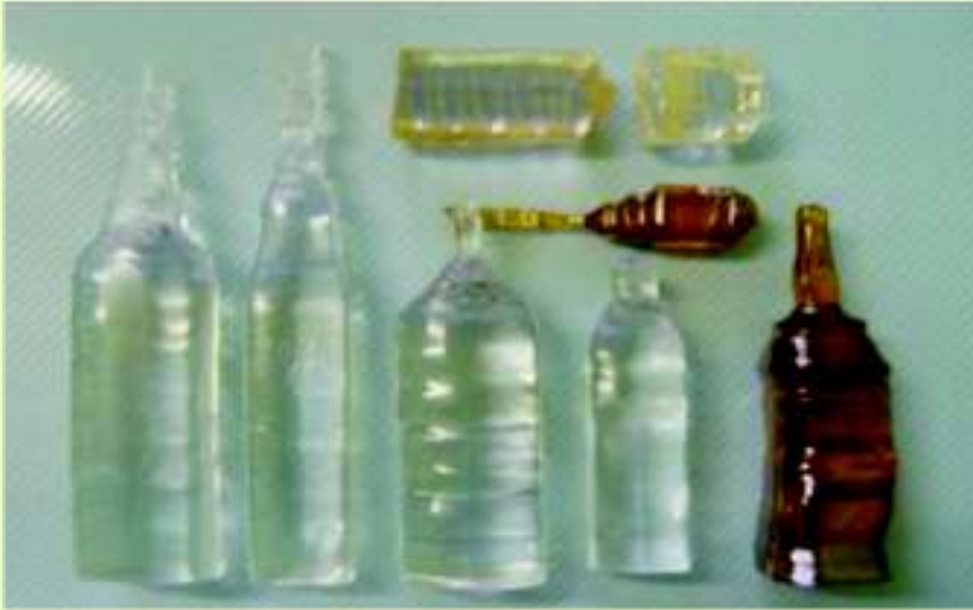
NaCl, LiNbO 3 , Bi 12 SiO 20 crystals grown using developed ADC puller
