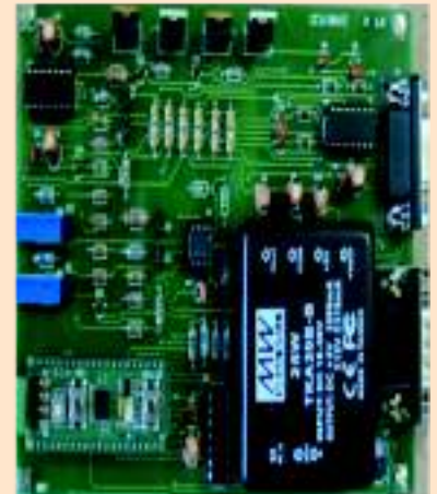
Wirelessly controlled ROHYTAM, Remote control chair, Dual Axis Servo controller card with RS485 interface
