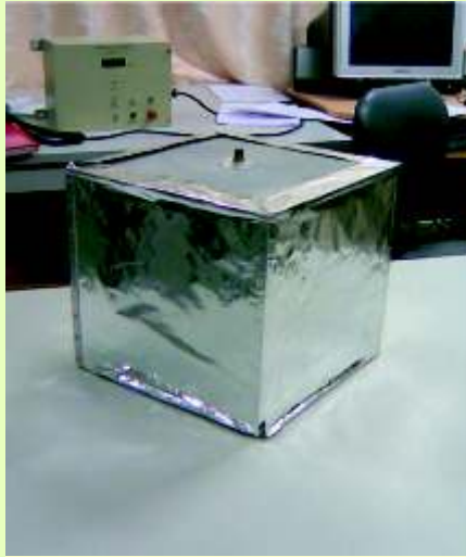
Thin walled Al Ionization Chamber
