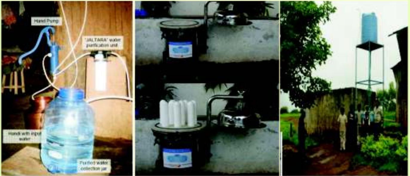
Rural adaptation of BARC developed community level solar photovoltaic driven Ultra-Filtration Water Purification units for villages without electricity
