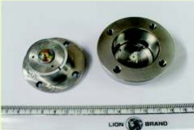
A diamond anvil cell with Be backing plates
