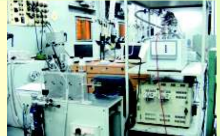
Analysis system with the gas chromatograph and the quadrupole mass spectrometer kept in the operating area of the hot cell
