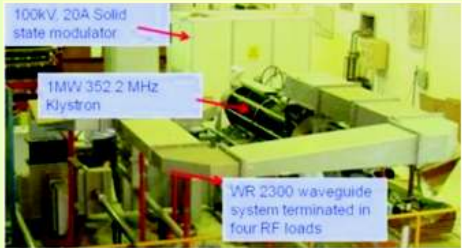
1MW pulsed test stand developed at RRCAT
