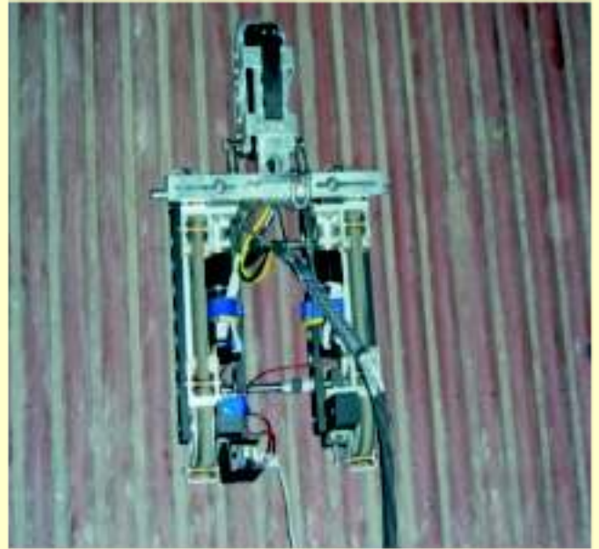
Field testing of magnetic crawler with EMAT
