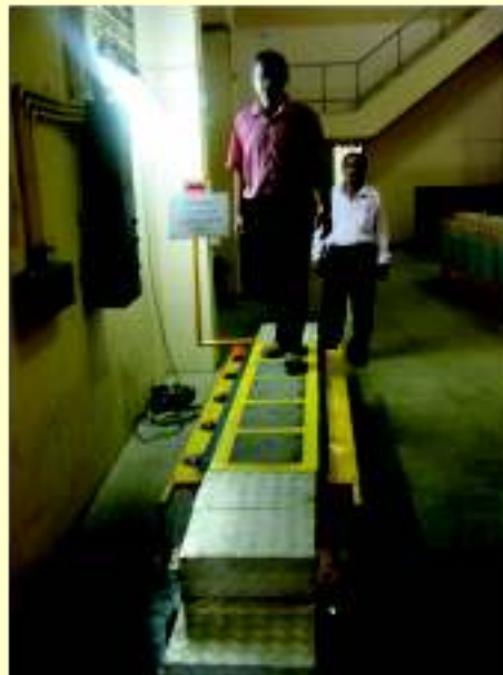
Foot Step Electric Converter platform
