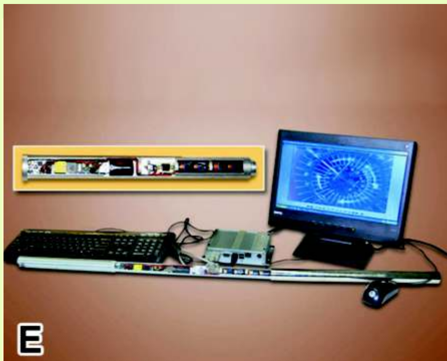
Modified borehole camera survey unit with CMOS image sensor
