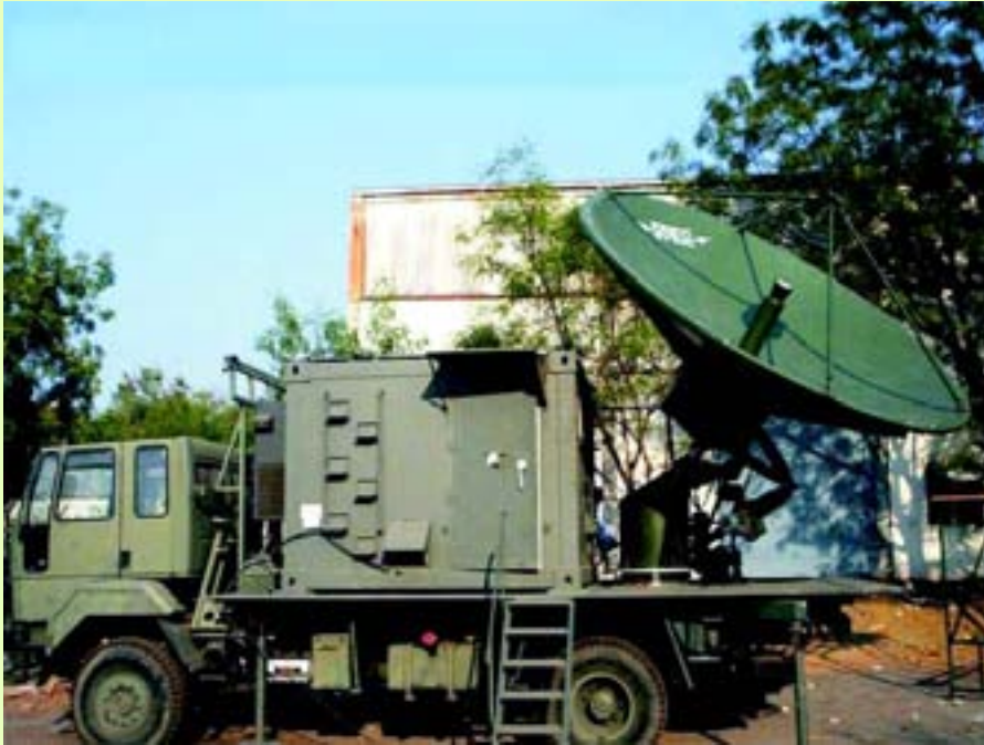
Mobile 3.8 m Data Dissemination Terminal developed by Electronics Corporation of India Limited.
