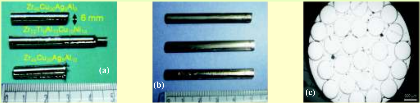
(a) Bulk metallic glasses (b) Composites of bulk metallic glass and tungsten fibres (c) Cross sectional view of the composite
