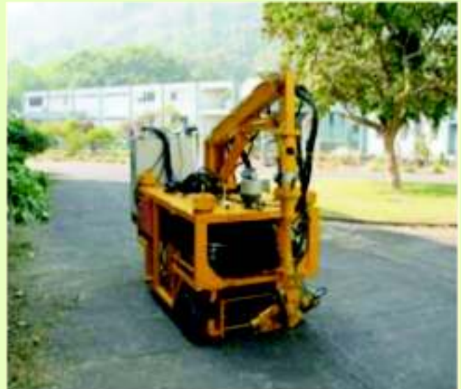
Wireless controlled ROHYTAM developed at Trombay
