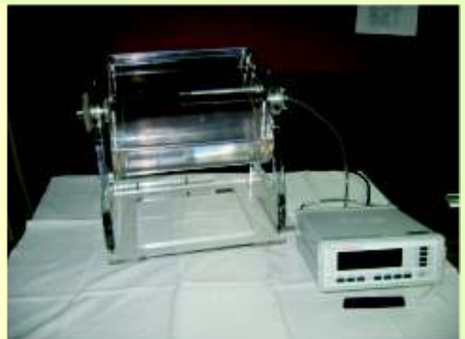
2D matrix ionization chamber system embedded Phantom with Farmer type ionization chamber for in the phantom to measures the composite dose the point dose verification in IMRT distribution for IMRT dose verification
