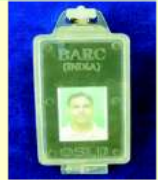
Optically Stimulated Luminescence Dosimeter Badge
