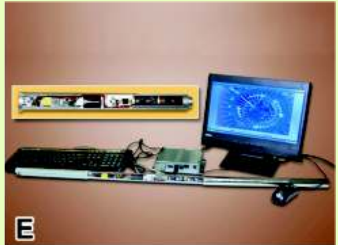
Modified borehole camera survey unit with CMOS image sensor
