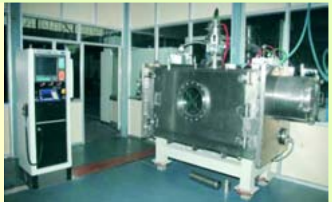
Indigenously fabricated Electron Beam Welding unit with imported gun and power supply
