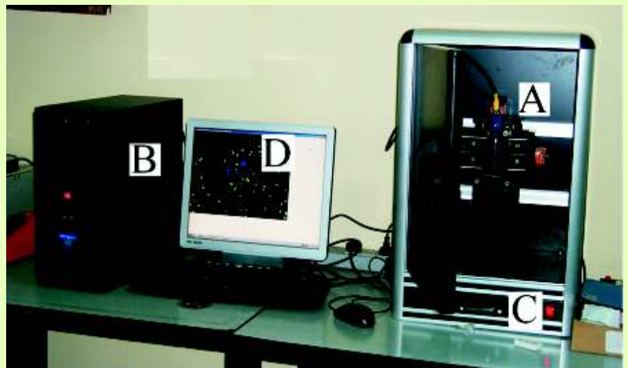
Image Analysis system analog CCD camera (A), Pentium P-IV PC (B). A sliding tray (C), image of tracks (D) is seen on monitor
