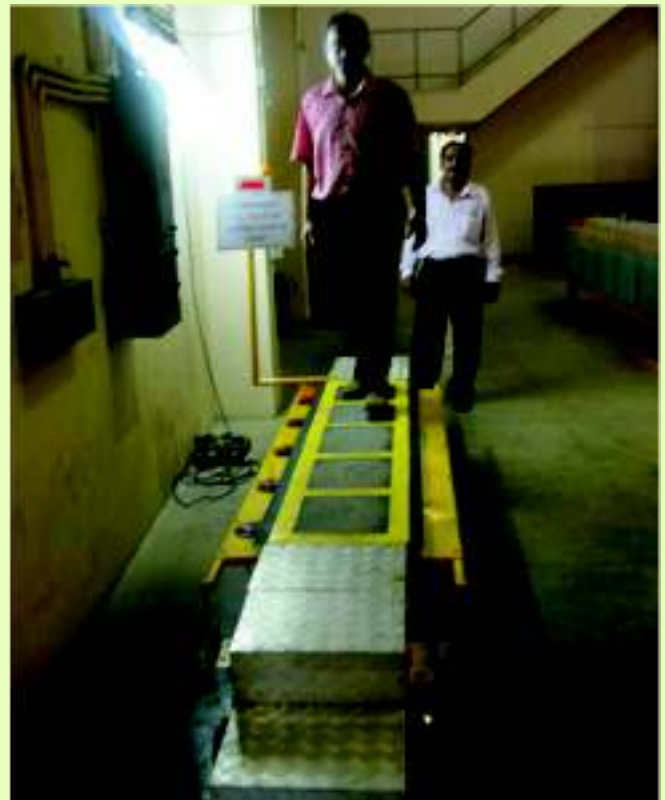
Foot Step Electric Converter platform developed at BARC
