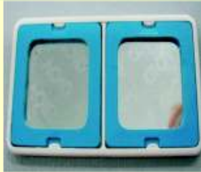
Personal badge dosimeter using DTPS/DRPS
