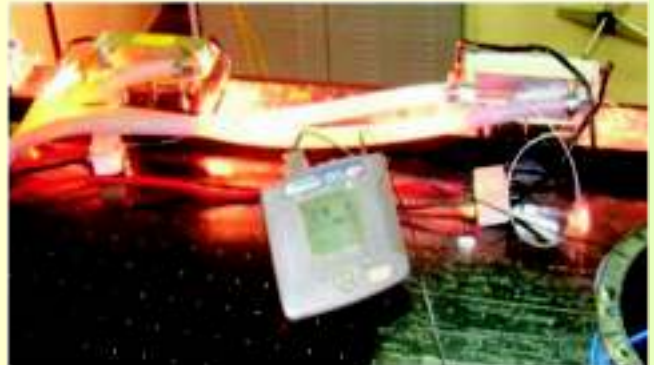
500W average power fibre coupled pulsed Nd:YAG laser
