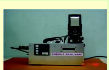
The Compact Aerial Radiation Monitoring System
