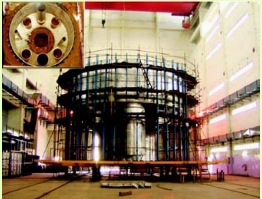
Inner vessel (Bhavini) of Prototype Fast Breeder Reactor
