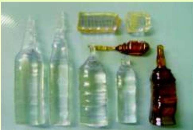
NaCl , LiNbO_3 , Bi_{12}SiO_{20} crystal grown using ADC puller developed inhouse by IGCAR
