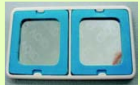
Personal badge dosimeter using DTPS/DRPS
