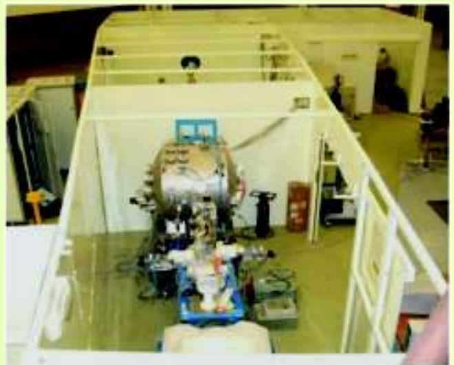
Indus-2 Synchrotron Radiation Beam Line with shielding hutch
