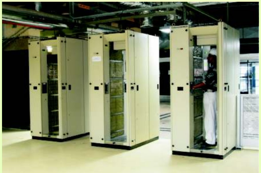
PC based whole body contamination monitor
