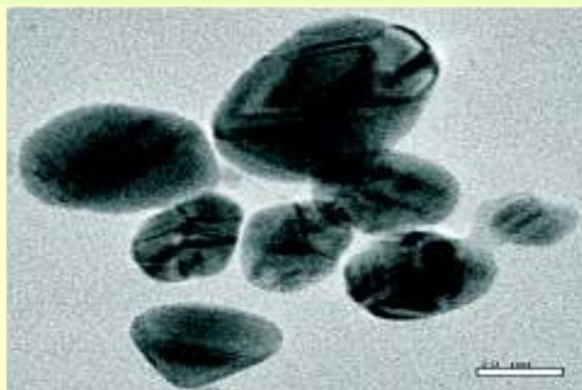
Synthesis of Ag nanoparticles from AgNO 3 using gum kondagogu ( Cochlospermum gossypium ), a natural biopolymer
