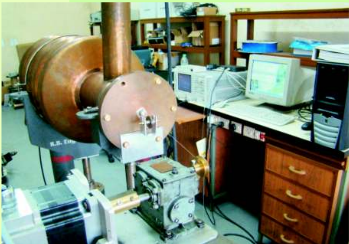
Bead-pull measurement set-up at VECC for 5-cell Linear Accelerator (LINAC) cavity
