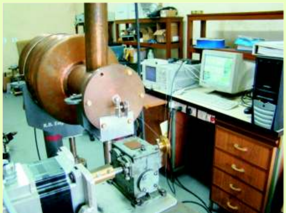
Bead-pull measurement set-up for 5-cell LINAC cavity
