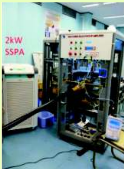
A 2 kW RF amplifier experimental set-up
