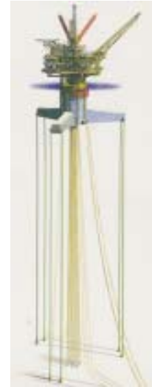
Figure 5 – Vertical Mooring System [17]
