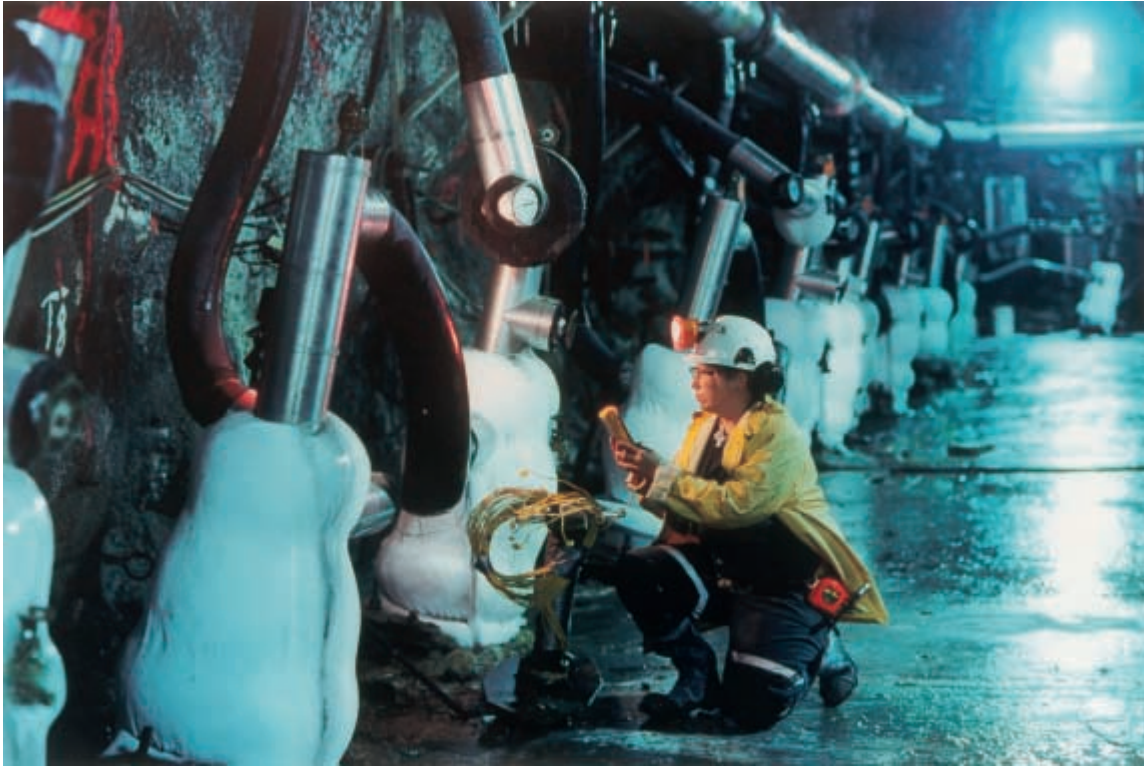
FIG. 30. Freeze chamber on the 530 m level of McArthur River underground mine, Saskatchewan, Canada.
