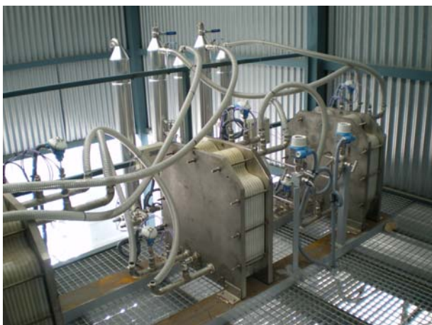
Figure 8.2 Scarab distillation membranes in the experimental facility built at the PSA-CIEMAT (Almería, Spain).
