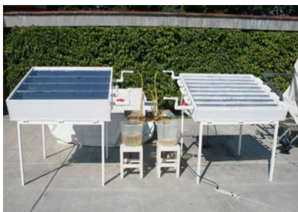
Figure 8.13 Comparison of CPC solar photoreactors with fixed catalyst, with 2 (right) and 1 (left) suns concentration ratio, CIE-UNAM
