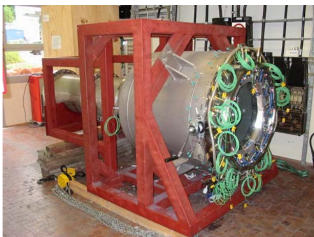
Figure 4.1. SOLREF reactor assembled at DLR Stuttgart and ready for shipping to WIS.
