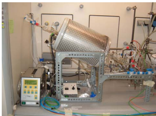
Figure 4.14. Lab rig for ageing tests: development of catalyst/substrate combinations for solar \text{SO}_3 reduction.
