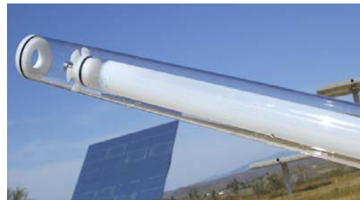
Figure 8.11 CPC SODIS reactor containing different immobilised catalyst configurations (left). Picture of "Uncoated external, \text{TiO}_2 coated internal" configuration before installing (right).
