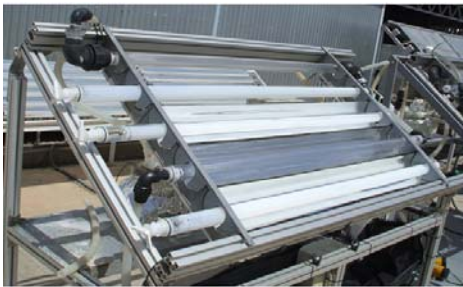
Figure 8.11 CPC SODIS reactor containing different immobilised catalyst configurations (left). Picture of "Uncoated external, \text{TiO}_2 coated internal" configuration before installing (right).
